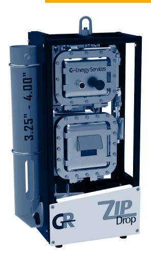
The ZipDrop optical remote ball dropper saves time and eliminates the need for personnel to work at heights or in the red zone to place a ball in the top of the wellhead. The unit is 38.5 in. long, 22 in. wide and 10.5 in. deep and weighs 125 lbm. The yellow ball hopper is available in four different ball size ranges:
