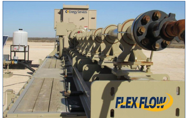
The Flex Flow horizontal pumping system drives a hydraulic jet pump downhole.
