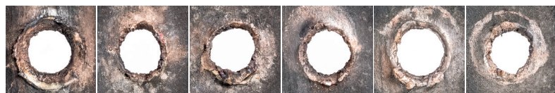
Entry holes created by StrykeZone XACT charges.
